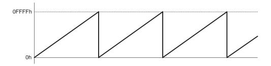
The TAIFG interrupt flag is set when the timer *counts* from 0FFFh to zero. Figure 11–5 shows the flag set cycle.
